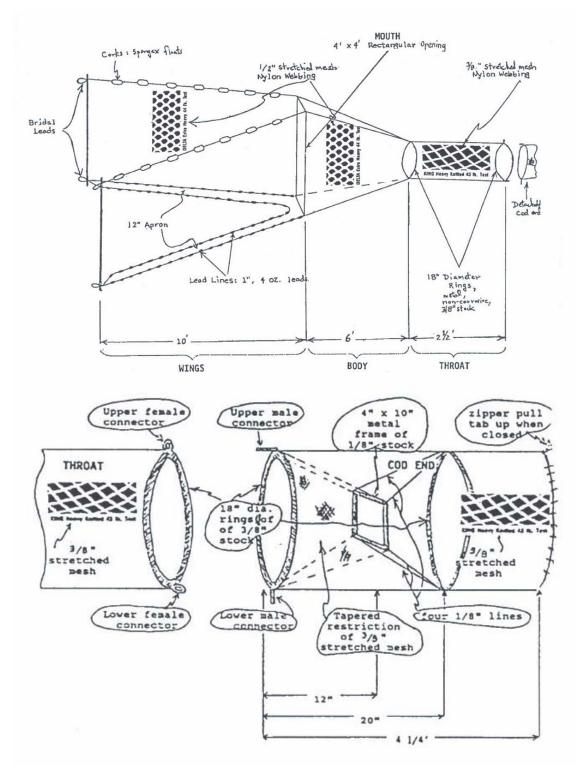
Figure 2. Diagram of fyke net used for sockeye salmon smolt emigration sampling on the Kvichak, Alagnak, and Nonvianuk Rivers, 2005.
