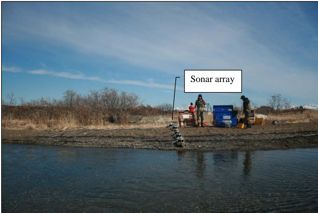
Photo 6. Sonar array staged for deployment on the Ugashik River, 2011.
